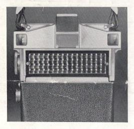
Super Kodak's photoelectric cell is mounted behind pressed multiple collective lenses (see at left). As the shutter speed is changed, a light-valve designed like a "Venetian blind" automatically varies the area exposed to light. The cell covers the same field as the main camera lens, and light falls on the two at an identical angle.
