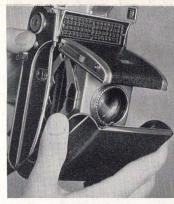
A touch of a button and a pull on the curved support bring the lens to picture-taking position. And a single movement locks it safely away.
