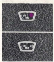
Signal of conspicuous color shows in shutter-speed scale, as warning to user, until shutter has been set—then it automatically disappears.
