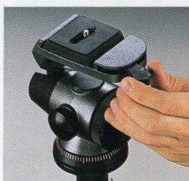
To release the Quick Plate, squeeze secondary safety lock and push lever forward at the same time.
