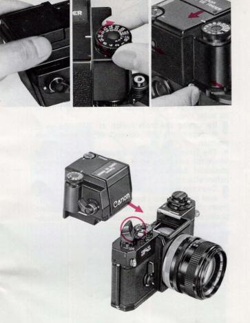
**6** Set the film speed scale on the Servo EE Finder at the film speed of the film to be used. Lift and turn the ring around the shutter speed dial. This can be performed more easily while pressing the center of the dial.
