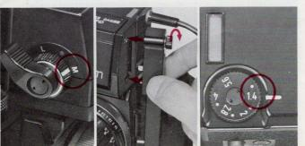
11 When the lens speed adjustment dial is turned, the f/stop scale of the meter reading window, slides and the lens speed is indicated just below the under-exposure warning mark as a maximum f/stop.
