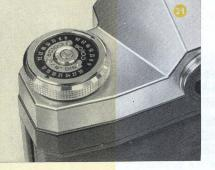
index mark of the outer ring points to the type and speed of the film in the camera (Fig. 31).
