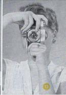
right hand the focusing mount (1). Use the left hand to support the CONTAFLEX from below. The illustrations on these pages show the various ways of holding the camera; so select the one that suits you best.
