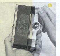
cassette with the exposed film. Be sure to remove immediately from the camera any fragments that might have come off the film.
