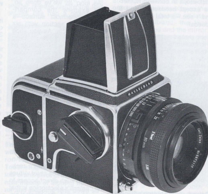
Evolutionary approach is evident in 2000FC's overall design. Most changes—multi-mode mirror, closer-focusing optics with more convenient controls—are for the better, but C/M's self-timer and T lock on shutter button got lost in the shuffle.
