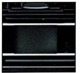
Titanium Electro-Mechanical Shutter In designing the LX. Pentax engineering craftsmen opted for a horizontally-run metal focal plane shutter to aid in keeping internal vibration at an absolute minimum, Titanium was selected as the material for the shutter curtains because of its greater durability and resistance to temperature extremes. For you, the photographer, this means reliability. accuracy and dependability even under the most difficult shooting situations.
