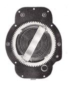
Press Graflex Shutter Control Mechanism
