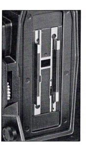
abrasion - resistant surface with good gliding properties. The gap formed between the front aperture plate and the back plate when the magazine is mounted prevents any appreciable frictional stress and thus ensures the best possible protection of the film. A small, spring-loaded pressure plate forming part of the magazine back plate presses the film into the flat position in the focal plane required for exposure.
