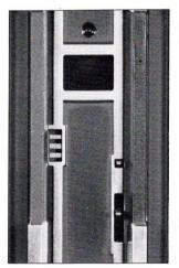
With this system, 4 bits per frame in a fixed relationship to the perforations of the film are exposed on the 2 mm wide sound track. The corresponding exposure apertures in front of the LEDs are located in the film channel of the 16 SR two frames below the gate.
