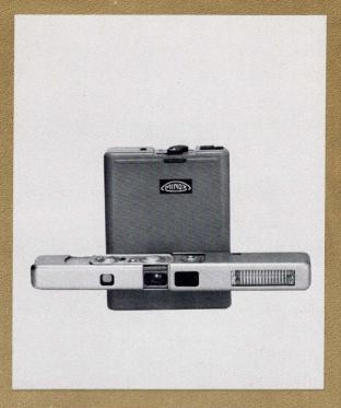
The Minox-Heliotron consists of a tiny (2%'') two ounce chrome-finish flash head containing the flash tube and ready light, and a separate, small  $(3 \times 4 \times 1'')$  ten ounce power pack with a built-in rechargeable nickel-cadmium battery which delivers up to 160 flashes on each full charge. The power pack can be recharged from any 110-117V AC outlet by means of the charger/power cord supplied with the outfit.
