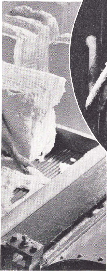
ABOVE—Drying purified cotton linters preparatory to their being used in the making of film base.
