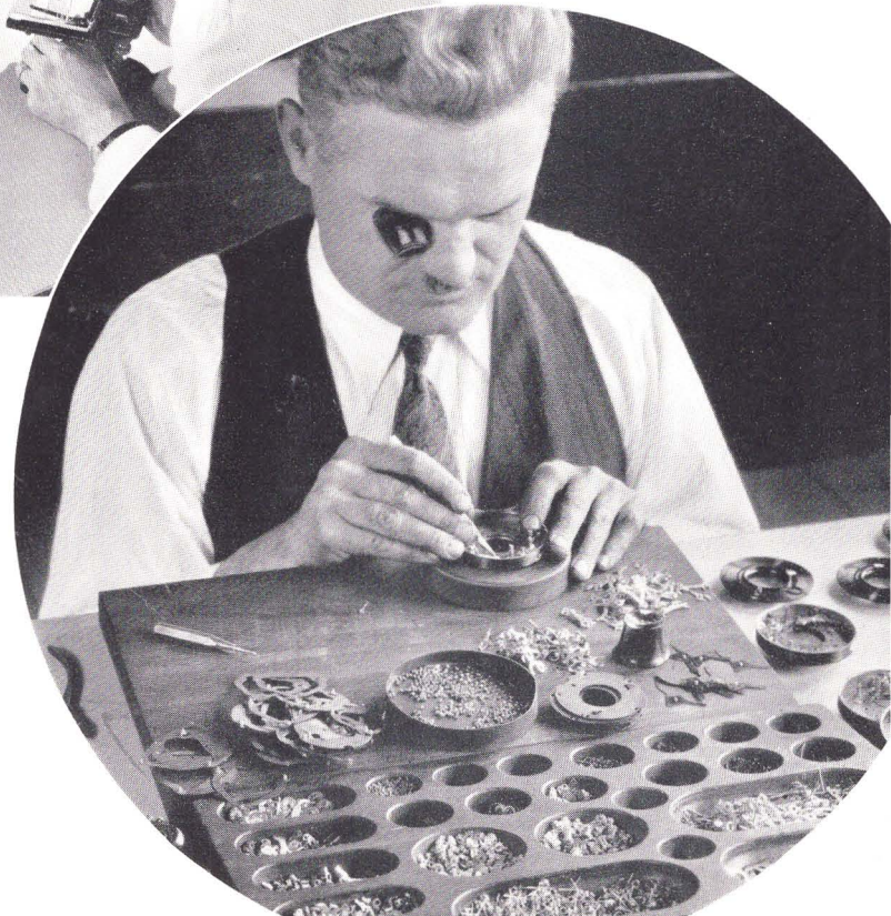
BELOW—Assembling automatic shutters: A job that requires the delicate handling of parts as minute as those found in the most expensive timepieces.
