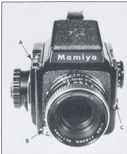
Front view shows dual shutter releases (A) and (B). Lower release has lock which acts to prevent both from being released; also has threaded receptacle for cable release. Lens bayonet latch (C) is on the right.
