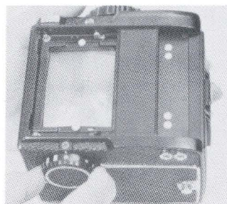
Set body shutter dial to dot-in-circle mark and mount meter finder; now meter's shutter dial takes over via terminals at right-hand top corner. Bottom right terminals provide sync.
