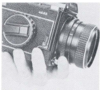
You can also trip shutter with left index finger. Camera body contour helps you hold camera firmly.
