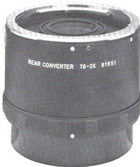
An ideal accessory for the 6x7 professional who needs telephoto lens versatility with the least amount of added bulk and weight. Doubles the effective focal length of Takumar and Pentax 6x7 telephotos of 135mm or longer (not including 500mm or 1000mm) yet adds only 2.4" (61mm) in length and 15.6 ounces (443g) in weight to ensure maximum handling ease. Super-Multi-Coated 6 element in 5 groups construction.
