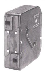
A 400' coaxial cassette mag is encased in the TGX-16 as part of the configuration of the camera. It's self-insulating and eliminates any possibility of light leaks or damage to the mag.
