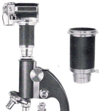
When mounted between the camera body and microscope, this adapter makes microscopic picture-taking extremely easy. The camera lens is taken off.
