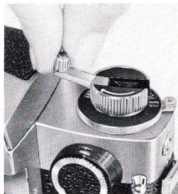
Flip the rewind crank on the rewind knob and wind in the direction of the arrow. At the end of the roll you will feel the resistance increase and then suddenly cease. Turn the rewind crank several more times to make certain the film has been entirely rewound.
