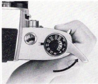
**Turn film advance lever several times to wind up the fogged portion of film**
