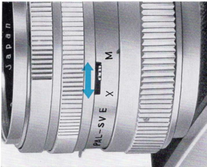
When using M-class flashbulbs, switch the sync selector lever to "M". Set the sync selector lever to "X" when using F-class flashbulbs or electronic flash unit.
