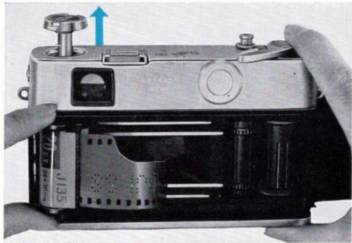
3. Fold out the crank-handle on the film rewind knob and turn it in the direction of the arrow. A slight resistance will be felt when the film pulls off the take-up spool, but continue winding the crank-handle.
