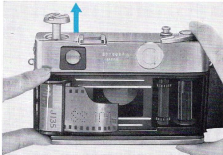
1. The rear cover will pop open when the rear cover lock on the edge of the camera base is pulled out.
