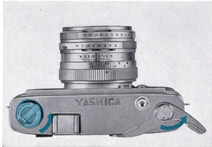
5. All the while during film loading, the exposure counter will register the letter "S" (Start). Release the shutter and wind the film advance lever alternately until the figure "1" appears in the counter window. (The exposure counter of the Lynx-14E automatically resets to "S" when the rear cover is opened.)
