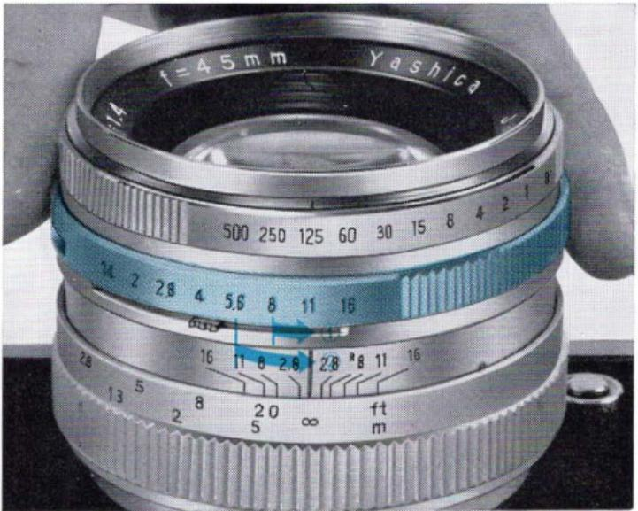
In order to obtain perfect exposure of the prime subject when shooting against light, it is necessary to give from twice to four times the normal exposure. The range of exposure adjustment in this case depends upon the intensity of the light in the background.
