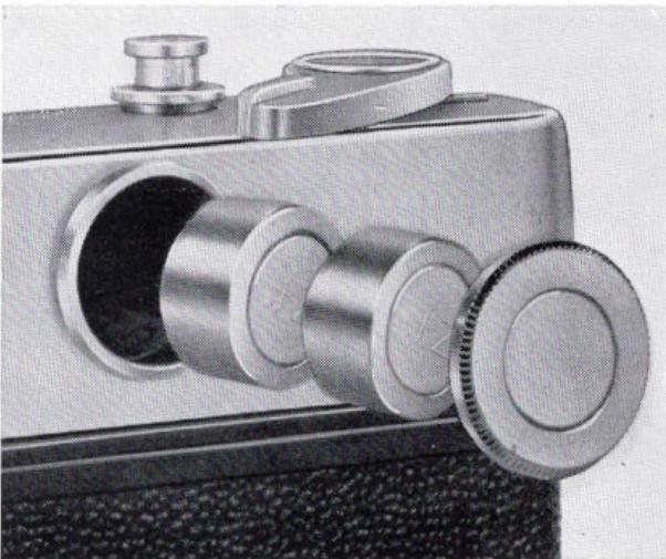
Open the battery compartment lid by turning it counter-clockwise. As illustrated, install two mercury batteries so that their plus (+) side faces towards you and close the lid securely.
