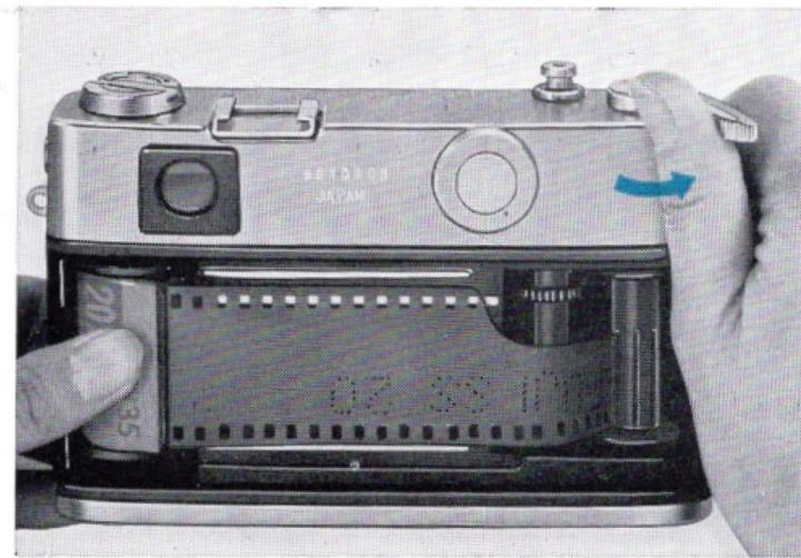
3. Draw out some length of the film from the cassette and introduce the tip of the film leader into one of the slots on the take-up spool.
