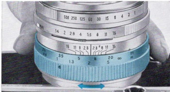
Focus adjustment is accomplished by turning the focusing ring while observing the image in the focusing spot in the center of the viewfinder field.
