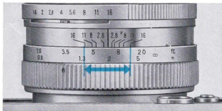
By depth of field, it is meant the range over which objects in the foreground and background appear acceptably sharp when the camera lens is focused on a subject at a given distance. The depth of field becomes more extensive when the lens aperture is closed to a smaller opening and likewise increases in proportion to the camera-to-subject distance.
