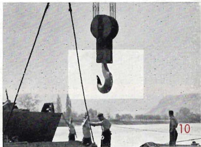
Coincidence of contours in combined view and rangefinder field
