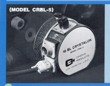
Crystalok is an extremely compact, lightweight control unit which, when added to an Arri 16-BL camera (with a standard universal motor), provides high precision crystal motor control. The unit also provides continuously variable speed control from 14 to 48 fps.
