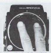
Six spring-loaded contacts within top section of SQ's lensmount mate with those on mounted lenses to transfer shutter-timing and exposure information to and from the camera circultry.
