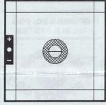
Bronica SQ's finder shows meter display area at left only when CdS meter finder is mounted. Entire LED array is shown for clarity, but only one symbol appears at a time in normal metering. Central focusing aids are large, easy to use; fine Fresnel outer area is very bright and contrasty.
