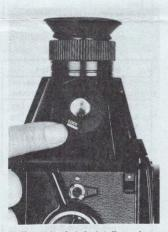
Pull out lock tab (at finger) on meter finder's shutter dial and "meter on" button above it can't be pressed in. It's a good safety feature, but we wish you could also lock meter on for extended shooting.
