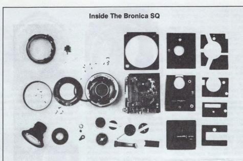
Basic stripdown of Bronica SQ shows amazingly simple construction for a 2<sup>1</sup>/<sub>4</sub> SLR, with a minimum of mechanical assemblies. This is made possible by an electronically controlled shutter and exposure info relay systems.
