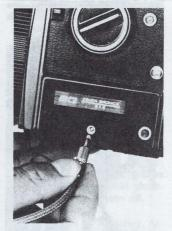
Threaded socket directly below body shutter dial accepts standard mechanical cable release. Note rubberized gripping surface which runs along camera bottom to other side.
