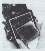
To replace viewing screen, just pop it into place (note one-way tab in proper position at back edge of screen unit) and move tabs forward so bars retain side tabs on screen.
