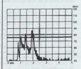
Although this camera's noise level peaks at 86 dB and includes three sound energy spikes to greater than 75 dB, its average noise output measures 75 dB, or slightly quieter than average for a 21/4 SLR. The results of these measurements were borne out in informal listening tests.
