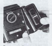
To remove film magazine insert dark slide, then press mag lock button in and lift it off starting at bottom.
