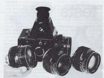
Here's the present system: Bronica SQ with 80mm f/2.8 Zenzanon lens, film magazine and CdS MF Finder S mounted. In front of camera from left to right are 50mm f/3.5, 105mm f/3.5 and 150mm f/3.5 Zenzanons. All are roughly similar in size and identical in control layout enabling fast familiarization and swift operation.
