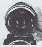
Studlike contacts on the back of SQ's lenses mate with those near top of body mount to transfer shutter timing and exposure info.
