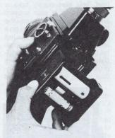
To load film line up arrow on film's backing with red arrow in insert and snap into position in mounted magazine.
