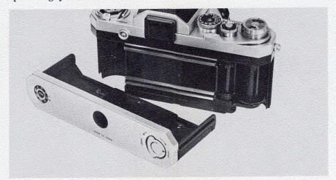
**BALL-BEARING FOCAL PLANE SHUTTER** offers speeds from 1 second to 1/100th, plus 'B' and 'T'. Speed selector dial does not rotate when shutter is wound or released. Shutter is thermally compensated to assure uniform, accurate speeds, even under temperature extremes. Extremely quiet in operation. Fast shutter curtain action miminizes elongation distortion, increases stop-action effectiveness.
