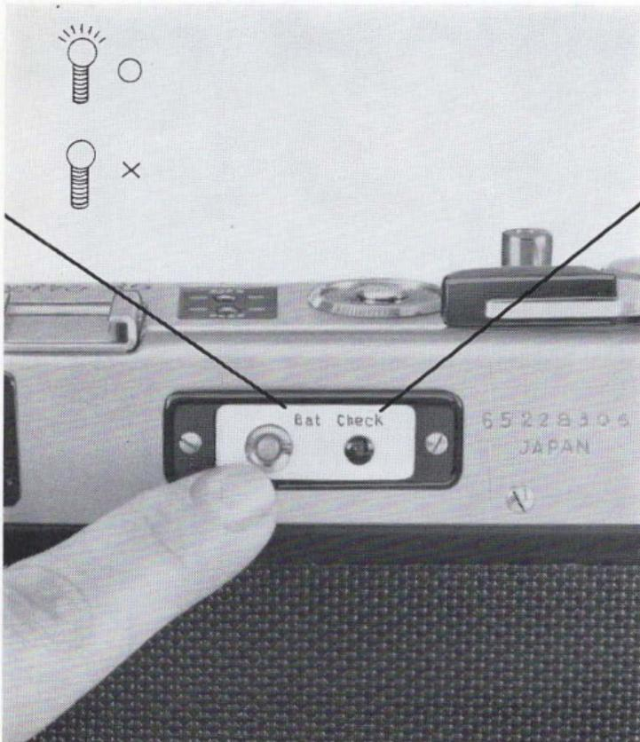
It is necessary to check the battery power before picture-taking, because sufficient battery power is required to obtain the correct exposure.
