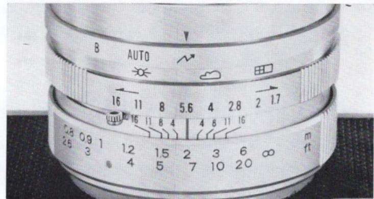
Set the flash mark  $\swarrow$  to the index line by turning the Exposure Control Ring. The shutter speed is set automatically at 1/30 sec. Electronic flash or flashbulbs can be used as the shutter speed is set at the X setting
