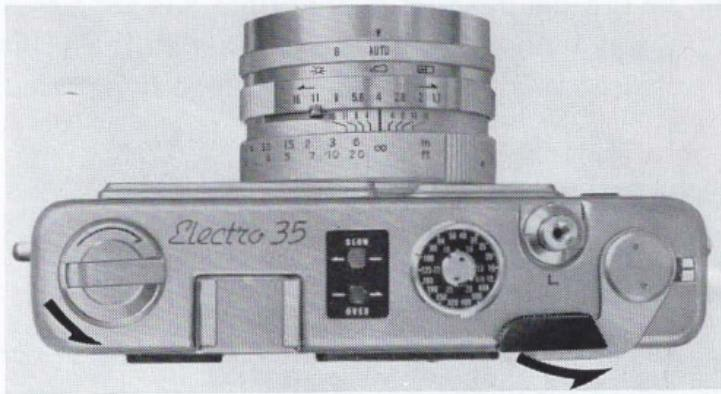
7 The Film Exposure Counter is automatically set to "S" (start) when the back cover is closed. Advance the film, press the Shutter Release Button and repeat until the figure "1" appears in the Exposure Counter Window. You are ready for your first exposure.
