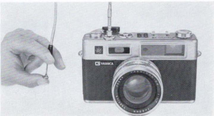
When the light is very weak, especially when you have to use a small stop, even the slowest shutter speed may be too short. In that case, you need time exposure. Set the Ring to B and press the release button. The shutter now remains open over the duration the shutter release button is depressed. For such time exposures, the camera must be mounted on a firm support such as a tripod.
