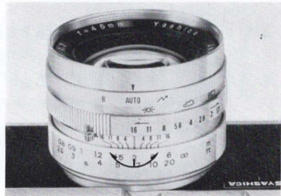
When you focus the camera on a subject, there is a certain distance in front and back of the subjects within which other objects will also appear sharp. This is known as the "Depth-of-Field" and it varies with the aperture. The smaller the aperture, the greater the Depth-of-Field.
