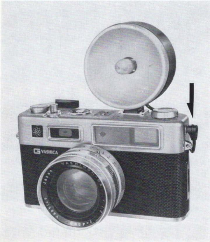
The electronic shutter is provided with B setting long exposure. However when you want to take pictures of moving subjects in dim light, the use of a flash gun is recommended.
