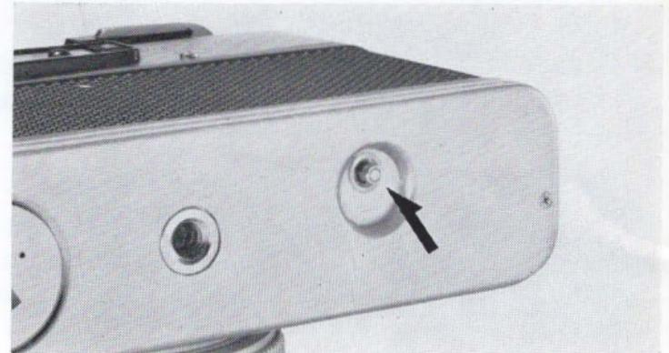
① After the last exposure (36 or 20), the film must be rewound into its cassette before removing it from the camera.
