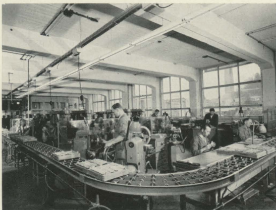
Fig. 11. The pressure-cast aluminium body of the Leica on the production line. Altogether 274 operations are carried out on it by milling, drilling and screw cutting machines.
