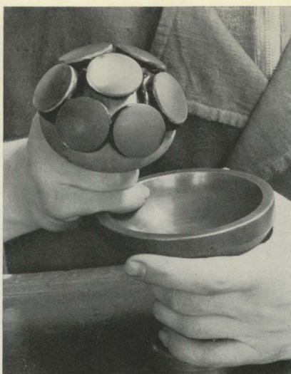
4 Grinding glass plates plane parallel. 5 The block of lenses is removed from the polishing tool. 6 The blocks of lenses are smoothed and polished on a multi-spindle polishing machine. Works photographs.
