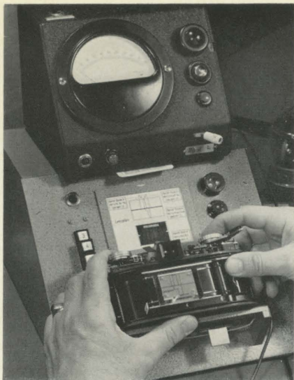
Fig. 15. Testing the adjustment and functioning of the flash synchronization of the Leicaflex.
