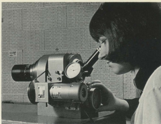
Fig. 10. Optical set-up of the LEICAFLEX-lenses is being checked.
