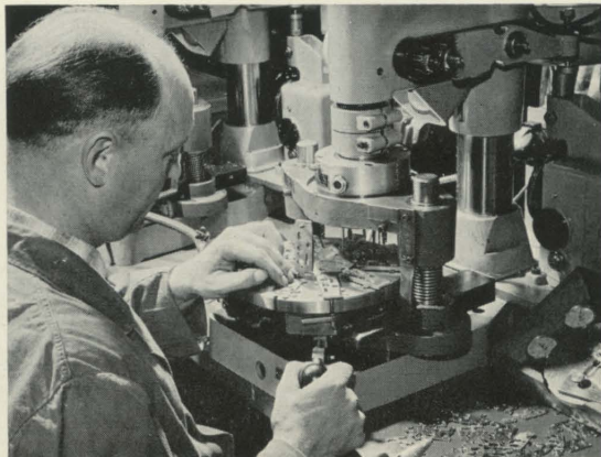
Fig. 3. Plates for the Leica shutter being drilled and countersunk on an automatic multi-spindle drilling machine.
