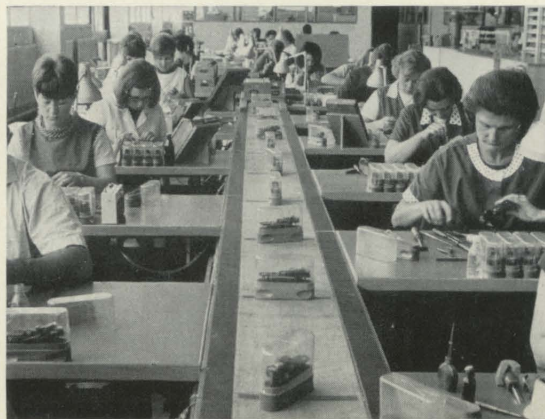
Fig. 8. Conveyor belt assembly of the camera shutter.
