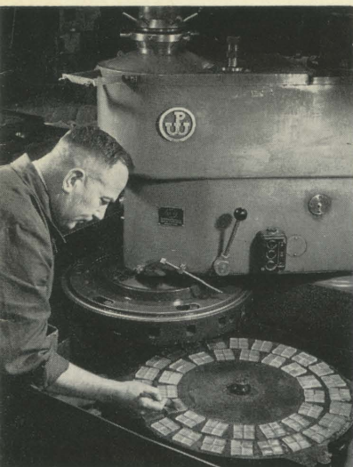
4 Grinding glass plates plane parallel. 5 The block of lenses is removed from the polishing tool. 6 The blocks of lenses are smoothed and polished on a multi-spindle polishing machine. Works photographs.
