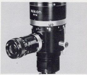
MICROFLEX PFM—Embodies its own image-forming optics, shutter mechanism and viewing system. Reduces overall magnification by one-half. Supplied with focusing ocular eyepiece for high-power photomicrography, and interchange-able ground-glass screen and 7x magnifier for low-power work. The screen also offers advantages in teaching and other group viewing applications.
