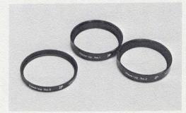
AUXILIARY CLOSEUP LENSES—Supplementary meniscus lenses in 52mm screwin mounts\* readily adapt camera for copying and closeup work. They require no exposure increase and do not interfere with automatic diaphragm action. Available in three progressively increasing powers: No. 0 (0.7 diopter), No. 1 (1.5 diopters) and No. 2 (3 diopters). May also be used in combination and in conjunction with extension tubes or bellows attachments.
