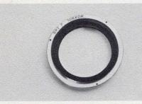
BR-2 LENS REVERSING RING Product No. 2630) Permits any lens with 52mm front thread\* to be mounted in reverse position on either Bellows Attachment. Provides optimum lens performance at reproduction ratios greater than 1:1. Also convenient for on-the-spot closeups when mounted directly on camera, with lens reversed.
