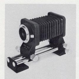
Model V/PB-5 (Product No. 2635) This is a simplified version of the PB-4, with one twin-track and minus the front standard movements. It offers the same range of magnifications, accepts the same lenses and both slide copying attachments.
