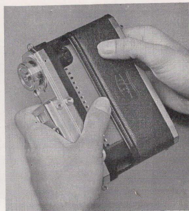
5. Film is wound on take-up spool until its perforations engage the teeth of the sprocket on both sides. Then back of camera is replaced.
