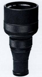
Focal Length 400mm Aperture Range: f4.5-f22 Angle of View · 6° 10' No. of Elements/Groups: 4/4 Coating: Multi-laver Nikon Integrated Coating Minimum Focus: 18.0' (5.5m) Diaphragm Type: Auto Filter Size: 122mm\* Dimensions: 5.3x10.8" (135x275mm) Weight: 4.2 lbs. (1900g) Other \* Accepts 52mm filters when used with Focusing Mount AU-1 Stopdown exposure measurement. Product No. 970
