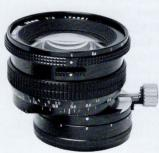
Focal Length: 28mm Aperture Range: f4—f22 Angle of View<sup>•</sup> 74° No. of Elements/Groups: 10/8 Coating: Multi-layer Nikon Integrated Coating Minimum Focus: 11.8″ (0.3m) Diaphragm Type: Manual Preset Filter Size: 72mm Dimensions: 3.1x2.7″ (78x67.5mm) Weight: 14.1 oz. (410g) Other<sup>•</sup> Supplied with Case. Product No.. 1022
