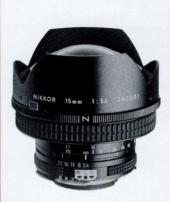
Focal Length 15mm Aperture Range: f5.6-f22 Angle of View 110° No. of Elements/Groups: 14/12 Coating Multi-layer Nikon Integrated Coating Minimum Focus: 11.8" (0.3m) Diaphragm Type: Fully Auto Filter Size: Built-in Skylight, Medium Yellow, Orange, and Red Filters Dimensions: 3.6x3.5" (92x88mm) Weight: 22.6 oz. (640g) Other Floating element system Product No. 1111 (Non-AI, 1011)
