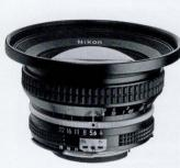
Focal Length: 18mm Aperture Range: f4—f22 Angle of View 100° No. of Elements/Groups: 13/9 Coating Multi-layer Nikon Integrated Coating Minimum Focus: 11.8" (0.3m) Diaphragm Type: Fully Auto Filter Size: Series 9\* Dimensions: 3.5x2.3" (89x58.5mm) Weight: 11 1 oz. (315g) Product No. 1113 (Non-Al, 1013)
