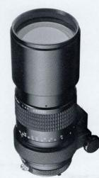
Focal Length: 300mm Aperture Range: f4.5—f22 Angle of View 8° 10' No. of Elements/Groups: 6/5 Coating Multi-layer Nikon Integrated Coating Minimum Focus: 13.0' (4.0m) Diaphragm Type: Fully Auto Filter Size: 72mm Dimensions: 3.1x8.0" (78.5x203mm) Weight: 40.2 oz. (1140g) Other · Built-In Telescopic Lens Hood Product No., 1170 (Non-AI, 1070)
