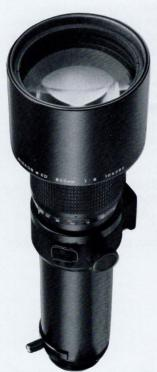
Focal Length: 800mm Aperture Range: f8-f32 Angle of View: 3° No. of Elements/Groups: 9/7 Coating: Multi-layer Nikon Integrated Coating Minimum Focus: 32.8' (10.0m) Diaphragm Type: Auto Filter Size: 122mm Dimensions: 5.2x18.1" (131.5x458.5mm) Weight: 8.4 lbs. (3800g) Other · Built-in Telescopic Lens Hood and tripod socket. Stopdown exposure measurement
