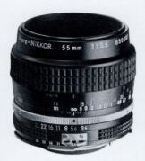
Focal Length: 55mm Aperture Range: f3.5—f32 Angle of View · 43° No. of Elements/Groups: 5/4 Coating Multi-layer Nikon Integrated Coating Minimum Focus: 9.5" (0.241m) Diaphragm Type: Fully Auto Filter Size: 52mm Dimensions: 2.6x2.5" (65.5x64.5mm) Weight: 8.3 oz. (245g) Product No. Lens only, 1140; with PK-13 ring, 1141 (Non-AI w/PK-3 Ring, 1040)
