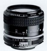
Focal Length 35mm Aperture Range: f2—f22 Angle of View· 62° No. of Elements/Groups: 8/6 Coating: Multi-layer Nikon Integrated Coating Minimum Focus: 11.8″ (0.3m) Diaphragm Type: Fully Auto Filter Size: 52mm Dimensions: 2.5x2.4″ (63.5x61mm) Weight: 9.9 oz. (280g) Product No., 1128
