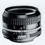
Focal Length 50 mm Aperture Range: f2.0—f16 Angle of View 46° No. of Elements/Groups: 6/4 Coating Multi-layer Nikon Integrated Coating Minimum Focus: 17 7" (0.45m) Diaphragm Type: Fully Auto Filter Size: 52mm Dimensions: 2.5x2.0" (63.5x50.5mm) Weight: 7.8 oz. (220g) Product No. 1136 (Non-AI, 1036)
