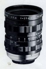
Focal length 25mm Aperture range: f1.4 to f22 No. of Elements/Groups. 7/5 Correction wavelength range: 400-700mm Picture angle: 28° (33° 22' with 1" vidicon) Vignetting: 0% (at f2.8) Distance scale: In meters and feet, from 0.6m (2 ft.) to infinity Image size: 16mm motion picture film and 1" vidicon format Weight: 140g (4.93 oz.) Diameter: 42mm (1.65") Length: 57mm (2.24") Rear mount: C mount  $(25.4 \text{mm}/1" \cdot 1/\text{P} = 32)$ Attachment size: 40.5mm
