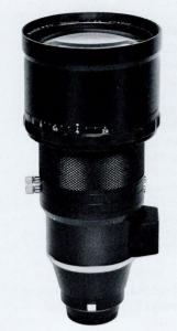
Focal Length: 300mm Aperture Range: f2.8-f32 Angle of View 8° 10' No. of Elements/Groups: 6/5 Coating Multi-layer Nikon Integrated Coating Minimum Focus: 13.0' (4.0m) Diaphragm Type: Manual Filter Size: 122mm Dimensions: 4.9x9.9" (125x251mm) Weight: 5.7 lbs. (2600g) Other · Built-in Telescopic Lens Hood. Stopdown exposure measurement Product No. 1298
