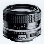
Aperture Range: f2.8—f22 Angle of View: 74° No. of Elements/Groups: 7/7 Coating Multi-layer Nikon Integrated Coating Minimum Focus: 11.8″ (0.3m) Diaphragm Type: Fully Auto Filter Size: 52mm Dimensions: 2.5x2.1″ (63.5x54mm) Weight: 8.5 oz. (240g) Product No. 1120 (Non-Al, 1020)
