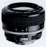
Focal Length 58mm Aperture Range: f1.2—f16 Angle of View: 40° 50' No. of Elements/Groups: 7/6 Coating: Multi-layer Nikon Integrated Coating Minimum Focus: 19.7" (0.5m) Diaphragm Type: Fully Automatic Filter Size: 52mm Dimensions: 2.9x2.5" (74x63mm) Weight: 17 1 oz. (485g) Other: Incorporates Aspheric Elements
