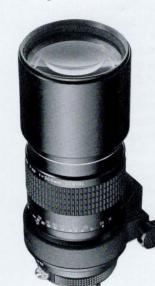
Focal Length 300mm Aperture Range: f4.5—f22 Angle of View 8° 10' No. of Elements/Groups: 6/4 Coating Multi-layer Nikon Integrated Coating Minimum Focus: 13.0' 4.0m) Diaphragm Type: Fully Auto Filter Size: 72mm Dimensions: 3.1x7.9" (78.5x200mm) Weight: 2.4 lbs. (1100g) Other Built-In Telescopic Lens Hood Product No., 1172 (Non-AI, 1272)
