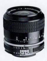
Focal Length: 28mm Aperture Range: f2-f22 Angle of View: 74° No. of Elements/Groups: 9/8 Coating: Multi-laver Nikon Integrated Coating Minimum Focus: 11.8" (0.3m) Diaphragm Type: Fully Auto Filter Size: 52mm Dimensions: 2.5x2.7" (64.5x68mm) Weight: 12.5 oz. (355g) Other: Floating element system Product No., 1119 (Non-Al, 1019)
