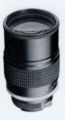
Focal Length: 180mm Aperture Range: f2.8—f32 Anale of View: 13° 40' No. of Elements/Groups: 5/4 Coating: Multi-laver Nikon Integrated Coating Minimum Focus: 70.9" (1.8m) Diaphragm Type: Fully Auto Filter Size: 72mm Dimensions: 3.2x5.6" (81x141mm) Weight: 29.3 oz. (830g) Other · Built-In Telescopic Lens Hood, Supplied with Case. Product No. 1165 (Non-Al, 965)
