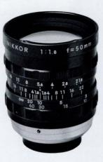
Aperture range: f1.8 to f22 No. of Elements/Groups: 4/4 Correction wavelength range: 400-700mm Picture angle: 14° 20' (17° with 1" vidicon) Vignetting. 0% (at f2.9) Distance scale: In meters and feet, from 1m (0.3 ft.) to infinity Image size: 16mm motion picture film and 1" vidicon format Weight: 175g (6.16 oz.) Diameter: 42mm (1.65") Length 52.5mm (2.07") Rear mount size: C mount  $(25.4 \text{mm}/1'' \cdot 1/\text{P} = 32)$ Attachment size: 40.5mm (P = 0.5mm)
