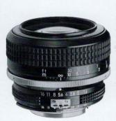
Focal Length 55mm Aperture Range: f1.2—f16 Angle of View· 43° No. of Elements/Groups: 7/5 Coating Multi-layer Nikon Integrated Coating Minimum Focus: 19.7" (0.5m) Diaphragm Type: Fully Auto Filter Size: 52mm Dimensions: 2.8x2.3" (72x58.5mm) Weight: 14.5 oz. (410g) Product No. 1138 (Non-Al, 1038)
