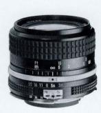
Focal Length: 28mm Aperture Range: f3.5—f22 Angle of View: 74° No. of Elements/Groups: 6/6 Coating Multi-layer Nikon Integrated Coating Minimum Focus: 11.8″ (0.3m) Diaphragm Type: Fully Auto Filter Size: 52mm Dimensions: 2.5x2.2″ (63x56mm) Weight: 8.5 oz. (240g) Product No. 1121 (Non-Al, 1021)
