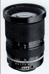
Focal Length: 35-70mm Aperture Range: f3.5—f22 Angle of View: 62°—34° 20' No. of Elements/Groups: 10/9 Coating: Multi-layer Nikon Integrated Coating Minimum Focus: 39.4" (1.0m) Diaphragm Type: Fully Auto Filter Size: 72mm Dimensions: 3.0 x 4.0" (75x101mm) Weight: 19.4 oz. (550g) Product No. To be announced Delivery: To be announced
