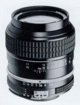
Focal Length: 105mm Aperture Range: f2.5-f32 Angle of View: 23° 20' No. of Elements/Groups: 5/4 Coating: Multi-laver Nikon Integrated Coating Minimum Focus: 39.4" (1.0m) Diaphragm Type: Fully Auto Filter Size: 52mm Dimensions: 2.6x3.1" (66x78mm) Weight: 15.3 oz. (435g) Other Snap-On Lens Hood supplied Product No.. 1156 (Non-Al, 1056)
