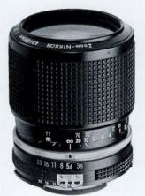
Focal Length: 43-86mm Aperture Range: f3.5—f22 Angle of View: 53°—28° 30' No. of Elements/Groups: 11/8 Coating · Multi-layer Nikon Integrated Coating Minimum Focus: 47.2" (1.2m) Diaphragm Type: Fully Auto Filter Size: 52mm Dimensions: 2.6x3.4" (65.5x85.1mm) Weight: 15.9 oz. (450g) Product No. 1181 (Non-AI, 1081)
