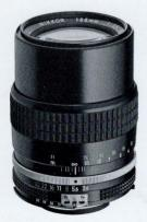
Focal Length: 135mm Aperture Range: f3.5-f32 Angle of View 18° No. of Elements/Groups: 4/4 Coating: Multi-layer Nikon Integrated Coating Minimum Focus: 51.2" (1.3m) Diaphragm Type: Fully Auto Filter Size: 52mm Dimensions: 2.6x3.5" (65x89.5mm) Weight: 14.1 oz. (400g) Other · Built-In Telescopic Lens Hood Product No. 1160 (Non-Al, 1060)
