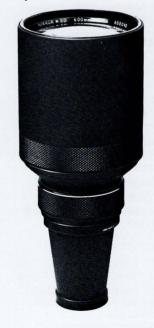
Focal Length 600mm Aperture Range: f5.6-f22 (automatic) Anale of View: 4° 10' No. of Elements/Groups: 5/4 Coating Multi-layer Nikon Integrated Coating Minimum Focus: 35.0' (11.0m) Diaphragm Type: Automatic and manual. Filter Size: 122mm\* Dimensions: Nikkor, 5.3x117" (135 mm) ED-Nikkor 5.2x12.3" (133 mm) Weight: Nikkor, 5.3 lbs. (2400g); ED-Nikkor 5.1 lbs. (2300g) Other: \*Accepts 52mm filters
