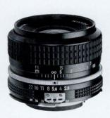
Focal Length 35mm Aperture Range: f2.8—f22 Angle of View· 62° No. of Elements/Groups: 6/6 Coating: Multi-layer Nikon Integrated Coating Minimum Focus: 11.8" (0.3m) Diaphragm Type: Fully Auto Filter Size: 52mm Dimensions: 2.5x2.1" (63.5x54mm) Weight: 8.5 oz. (240g) Product No.. 1127 (Non-Al, 1027)
