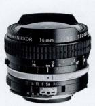
Focal Length: 16mm Aperture Range: f3.5—f22 Angle of View<sup>.</sup> 170° No. of Elements/Groups: 8/5 Coating: Multi-layer Nikon Integrated Coating Minimum Focus: 11.8″ (0.3m) Diaphragm Type: Fully Auto Filter Size: Built-in Medium Yellow, Orange, Red, and Clear filters Dimensions: 2.7x2.4″ (68x60.5mm) Weight: 11.5 oz. (330g) Product No.: 1109
