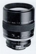
Focal Length: 135mm Aperture Range: f2—f22 Angle of View: 18° No. of Elements/Groups: 6/4 Coating. Multi-layer Nikon Integrated Coating Minimum Focus: 51.2" (1.3m) Diaphragm Type: Fully Auto Filter Size: 72mm Dimensions: 3.2x4.1" (81x103mm) Weight: 30.3 oz. (860g) Other: Built-In Telescopic Lens Hood Product No. 1159
