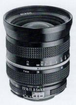
Focal Length 28-45mm Aperture Range: f4.5—f22 Angle of View· 74°—50° No. of Elements/Groups: 11/7 Coating: Multi-layer Nikon Integrated Coating Minimum Focus: 23.6″ (0.6m) Diaphragm Type: Fully Auto Filter Size: 72mm Dimensions: 3.0x3.6″ (75x91mm) Weight: 15.5 oz. (440g) Product No. 1180 (Non-Al, 1080)
