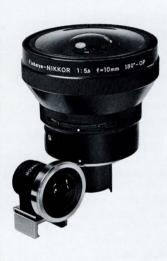
Focal Length: 10mm Aperture Range: f5.6—f22 Angle of View: 180° No. of Elements/Groups: 9/6 Coating: Nikon standard coating Minimum Focus: Fixed Diaphragm Type: Manual Filter Size: Built-in Skylight, Med. Yellow, Dark Yellow, Dark Orange, Red, and Light Green Filters Dimensions: 3.3x4.1" (84x105mm)
