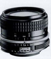
Focal Length: 24mm Aperture Range: f2.8—f22 Angle of View 84° No. of Elements/Groups: 9/9 Coating: Multi-laver Nikon Integrated Coating **Minimum Focus:** 11.8" (0.3m) Diaphragm Type: Fully Auto Filter Size: 52mm Dimensions: 2.5x2.2" (63x55mm) Weight: 9.5 oz. (265g) Other Floating element system Product No., 1116 (Non-Al, 1016)
