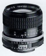
Focal Length: 85mm Aperture Range: f2—f22 Angle of View<sup>.</sup> 28° 30' No. of Elements/Groups: 5/5 Coating Multi-layer Nikon Integrated Coating Minimum Focus: 33.5" (0.85m) Diaphragm Type: Fully Auto Filter Size: 52mm Dimensions: 2.5x2.4" (63.5x60.7mm) Weight: 15.2 oz. (430g) Product No.. 1151 (Non-Al f1.8, 1051)
