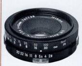
Focal Length: 45mm Aperture Range: f2.8—f32 Angle of View<sup>.</sup> 50° No. of Elements/Groups: 4/3 Coating Multi-layer Nikon Integrated Coating Minimum Focus: 31.5" (0.8m) Diaphragm Type: Fully Auto Filter Size: 52mm Dimensions: 2.5x1.2" (64x31mm) Weight: 6.0 oz. (170g) Other<sup>.</sup> Guide Number Scale 32-320 Product No.. 920
