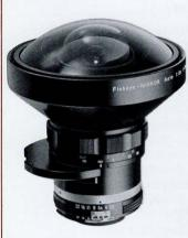
Focal Length 8mm Aperture Range: f2.8-f22 Angle of View 180° No. of Elements/Groups: 10/8 Coating: Multi-layer Nikon Integrated Coating Minimum Focus: 11.8" (0.3m) Diaphragm Type: Fully Auto Filter Size: Built-in Skylight, Med. Yellow, Dark Yellow, Orange and Red Filters Dimensions: 4.8x5.5" (123x140mm) Weight: 35.3 oz. (1.0kg) Product No. 1102 (Non-AI, 226\*)
