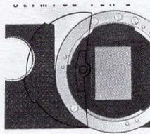
10) Unique *rotary* titanium focal plane shutter makes it possible to have full synchronization at *all* speeds. This is not possible with most 35mm full frame cameras because of shutter design limitations.
