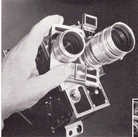
Rotating the turret brings "stand-by" lens into position. Only a simple turn is required.
