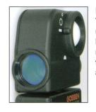
Flat diffuser: The flat position is used for measuring luminance, or for measuring light on flat objects, such as artwork.
