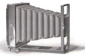
A N inexpensive, reliable view camera for those who do not require extra long bellows capacity. It is especially adapted for interior work as it focuses from the rear only, and the back may be moved as close to the front as desired so that extreme wide angle lenses may be used.
