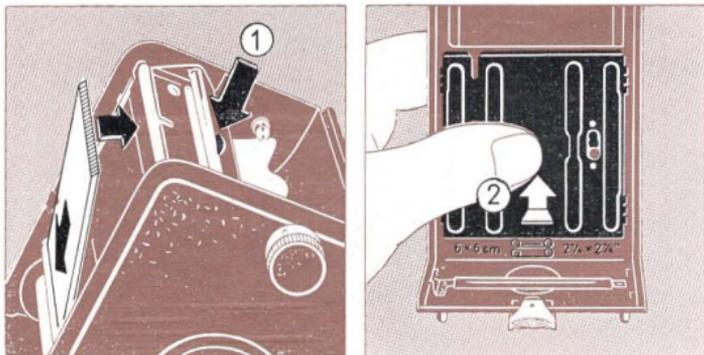
**To insert the flat glass:** open camera, and tilt forward. Slide glass with beveled edge under upper retaining bar of the film gate, let glass plate snap into position and secure by pressing bar ①. The beveled edges are held by the retaining bars of the film gate. To remove: turn camera upside down, press retaining bar ① and let glass drop into your hand.
