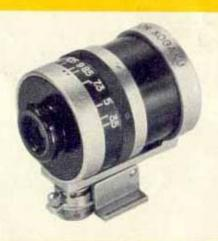
VARIFOCAL VIEW FINDER. "Zoom" type finder that magnifies image in proportion to focal length of lens for which it is set. Compensates for parallax. For use with 35mm to 135mm lenses. Available for Nikon or Leicu. Leather case supplied.
