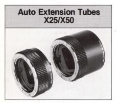
These extension tubes are attached between the lens and camera body for making ultracloseups and have tube lengths of 25mm and 50mm, respectively. Used with the 55mm normal lens, the X25 provides one-half life size images while the X50 produces life-size results. Focusing is easy because of the full-aperture, automatic function.
