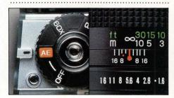
The AX-1 uses an aperture-priority AE system to make operation as simple as possible. For correct exposure all you have to do is set the shutter control dial to "AE" and select the desired aperture. The electronic circuitry automatically calculates and sets the required shutter speed. This system enables full control of depth-of-field because of the aperturepriority feature. Yet shutter speeds can also be controlled by merely changing the aperture as required.
