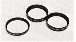
AUXILIARY CLOSEUP LENSES – Supplementary meniscus lenses in 52mm screw-in mounts\* readily adapt Nikon F for copying and closeup work. They require no exposure increase and do not interfere with automatic diaphragm action. Available in three progressively increasing powers: No. 0 (0.7 diopter), No. 1 (1.5 diopters) and No. 2 (3 diopters). May also be used in combination and in conjunction with extension tubes or bellows attachments.
