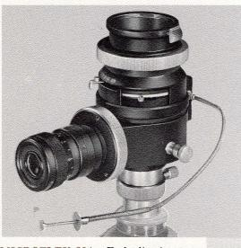
**MICROFLEX 804** — Embodies its own image-forming optics, shutter mechanism and viewing system. Reduces overall magnification by one-half. Supplied with focusing ocular eyepiece for high-power photomicrography, and interchangeable ground-glass screen and 7x magnifier for low-power work. The screen also offers advantages in teaching and other group viewing applications.
