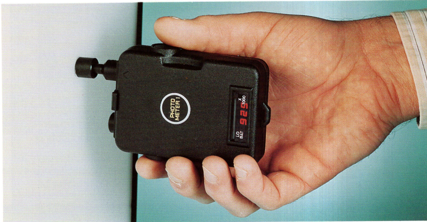
With the Fiber Optic Probe PM10, the PhotoMeter 1 or LX will give pin-point luminance readings
