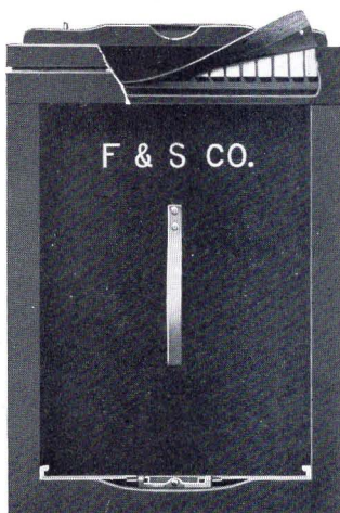
Graflex Plate Holder Showing Cut-off
