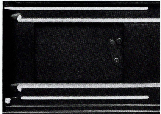
The electronically-controlled, quartz-timed automatic shutter of the FX-D.
