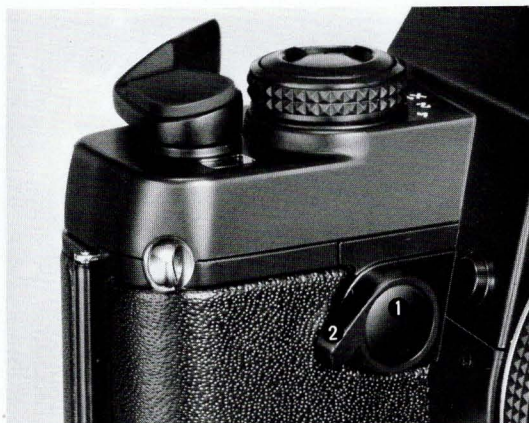
Pressing the Exposure Check Button lights the LED exposure display system for 10 seconds ①. An AE Lock Lever can be used to 'freeze' exposure values ②.
