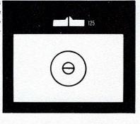
**2-second and 4-second exposures** Needle centered with shutter set at "B" indicates need for 2-second exposure; with shutter at "T," 4-second exposure.
