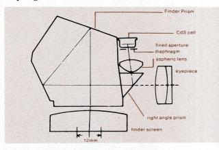
"Center-weighted" response FTN meter system receives about 60% of its exposure information from circular 12mm area in center of screen. From this area outward, meter
