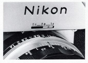
**Cross-coupled** Either the aperture ring or the shutter speed dial may be used to center the meter needle, visible in the finder and in the window on top of the FTN housing. Selected shutter speed is also visible in the finder. Auto-Nikkor lenses remain wide open during exposure setting, maintaining full advantage of automatic diaphragm action. FTN also permits stop-down measurements, with non-automatic
