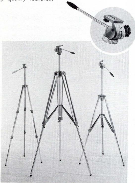
**HYDRONALIUM ALLOY.** Leg sections are made of sturdy, corrosion-resistant Hydronalium proven in hundreds of thousands of Linhof Precision tripods; each section is ground, polished and anodized to a smooth finish which keeps hands and clothing free from smudges. Hydronalium alloy combines lasting sturdiness with surprisingly light weight.
