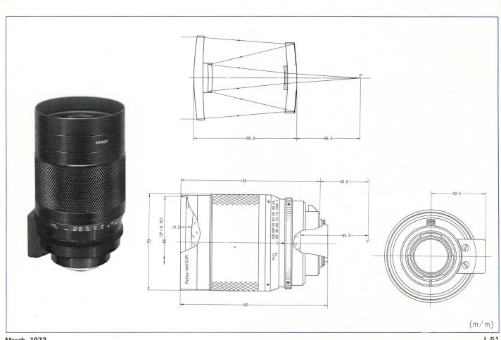
This is a very compact, lightweight super telephoto lens of the catadioptric type. Despite its 1000mm focal length, overall length is only 238mm. It weighs 1.9kg.
