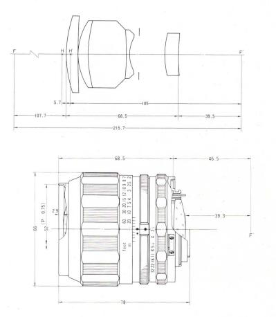
With a large aperture of f/2.8, this 135mm telephoto lens is well corrected for all aberrations and produces excellent resolution and high contrast even at full lens opening.
