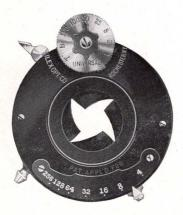
THIS shutter is strictly automatic in action and does not require setting. It may be operated either by finger-lever or bulb. The entire mechanism is controlled by one dial operating in either direction. It is the fastest speed automatic shutter ever produced, having a speed of  $\frac{1}{150}$ th second, which is fast enough for most purposes, and also has all intermediate speeds down to one full second in addition to "Time and Bulb."
