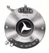
It has a three-blade, star-shaped light opening, giving a full, even illumination to plate or film, instead of the two-blade arrangement, opening from the center which gives a greater light exposure in the center and an uneven full illumination.
