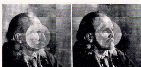
When double image (left) is superimposed (right) the object is in exact focus.
