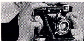
Moving milled wheel with one finger adjusts range-finder and brings lens to sharpest focus.
