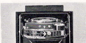
Figures on lens and shutter mounts, visible from above, show distance focused and depth of focus.
