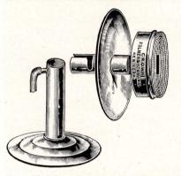
The Crown Flash Lamp is so constructed that the magnesium powder is stored in the body of the lamp and blown up through the center of flame, thoroughly consuming it and producing a powerful light. The head of lamp is filled with lampwick, saturated with alcohol. This gives a large flame, which is very essential in a perfect flash lamp.
