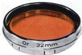
which otherwise might easily come out too dark, and the Or filter will even suppress freckles to a very large extent. Filter factor:  $5\times$ , when setting on light values 2.5 LV less.
