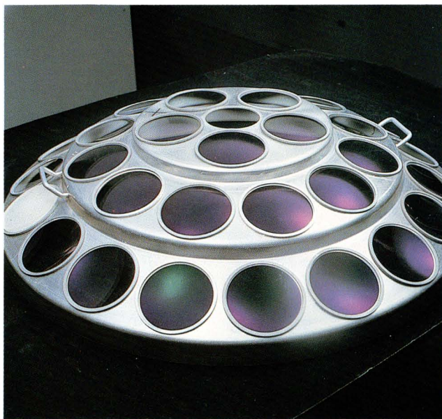
NIC is applied to elements loaded into a jig.
