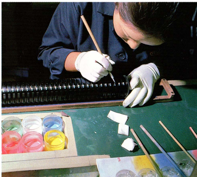
Hard painting of color-coded aperture numbers
