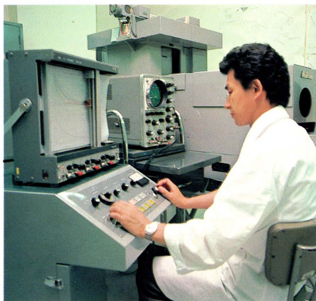
Nikon-produced MTF testing apparatus
