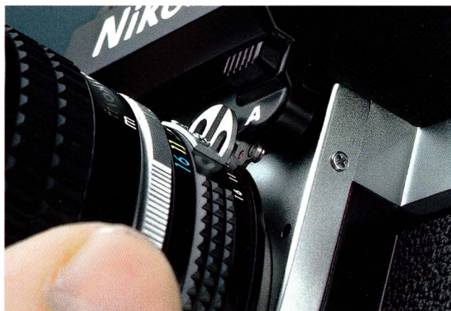
As soon as the lens is mounted, the maximum aperture is automatically indexed.
