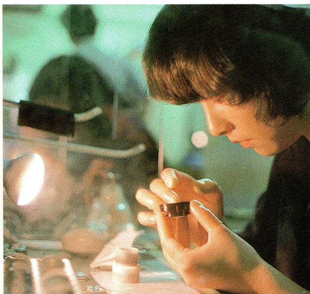
Placing a lens element into its retaining ring
