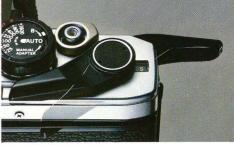
**Quick Action Wind-On Lever** Another example of the OM-10's attention to details, the film advance lever is carefully shaped to be unobtrusive but instantly accessible. A convenient feature lets you advance the film by repeated small movements, or by a quick flick over the short 130° winding angle. The 30° pre-advance angle lets you keep the lever open for fast repeat shots. tip Control System
