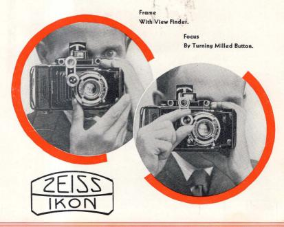
This is achieved by the reflecting end-surfaces of a glass rod and by two prismatic lenses arranged in front of one of the reflecting surfaces. Turning the milled button revolves the lenses and at the same time displaces the front element of the Tessar objective inward or outward, thereby focusing the camera.
