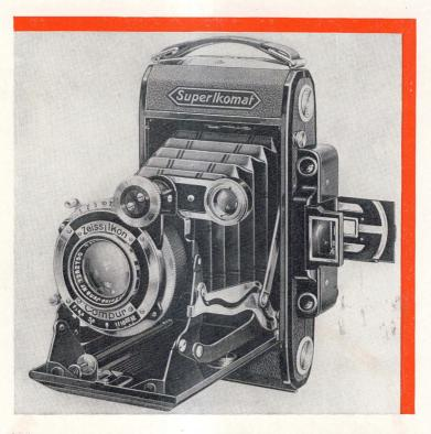
Pressing a button automatically opens camera and optical view finder. Swing out that part of the distance meter which is mounted above the lens and with the view finder frame your scene. Now look through the distance meter and turn the milled button as illustrated on pages 4 and 5. When you have coincidence your lens is focused,—critically sharp and ready for a perfect shot.
