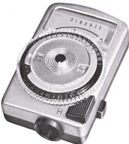
Sekonic Micro-Leader is more than 150 times as sensitive as conventional meters. Super-sensitive CdS makes it possible to get measurements of incredibly low light. Match-The-Needle system enables you to read exposure settings very easily and correctly. Battery checker is built in.
